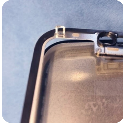
Poor display installation
